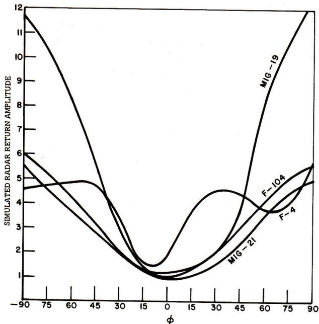
Fig. 2. Simulated radar return amplitude at given frequency as function of orientation.
