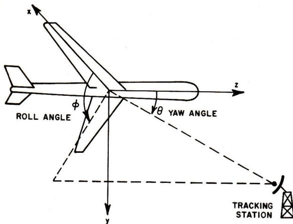
Fig. 1. Coordinate system to represent aircraft orientation.
