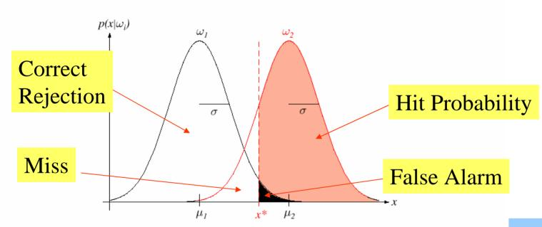
When no signal present:  $p(x/\omega_1) \sim N(\mu_1, \sigma^2)$
