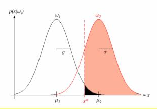
When no signal present:  $p(x/\omega_1) \sim N(\mu_1, \sigma^2)$
