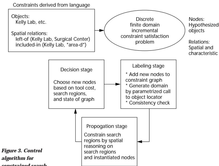
**Figure 3. Control algorithm for constrained search.**
