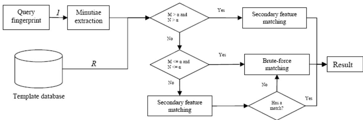
Figure 2.1.2: Multi-path Matching Schematic Flow.
