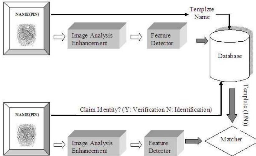
Figure 1.1.1: Schematic diagram of Fingerprint recognition Systems.
